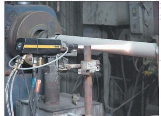
HVOF coatings can improve wear resistance and part life
