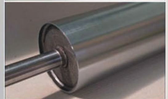
Chrome-plating to reinstate the surface
