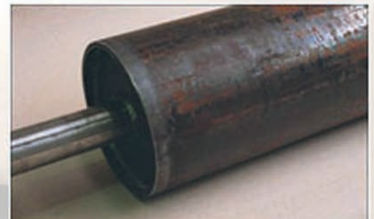
HVOF coatings can improve wear resistance and part life
