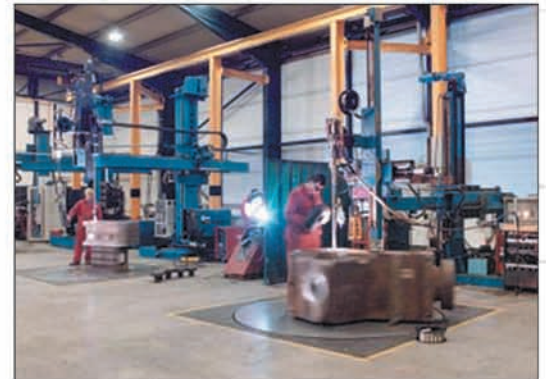
TIG welding to build up lost material
