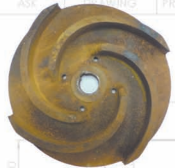
"Old" materials suffering from corrosion
